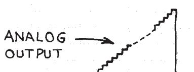
OUTPUT IS A STEPPED VOLTAGE. APPLICATIONS INCLUDE ANALOG-TO-DIGITAL CONVERSION AND WAVEFORM SYNTHESIS.
