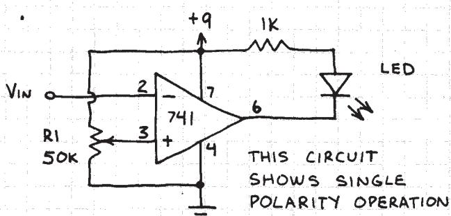
R1 SETS THE VOLTAGE DETECTION THRESHOLD (UP TO +9V). WHEN  $V_{IN}$  EXCEEDS THE THRESHOLD (ALSO CALLED THE REFERENCE), THE LED GLOWS.
