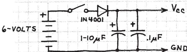
THE DIODE DROPS THE BATTERY VOLTAGE TO A SAFE LEVEL. BOTH CAPACITORS SHOULD BE INSTALLED ON THE TTL/LS CIRCUIT BOARD. CIRCUITS WITH LOTS OF TTL/LS CHIPS CAN USE LOTS OF CURRENT. USE A COMMERCIAL 5 VOLT LINE POWERED SUPPLY TO SAVE BATTERIES. OR MAKE YOUR OWN. (SEE THE 7805 ON PAGE 94.)
