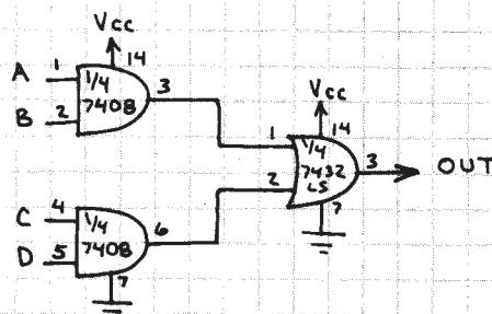
OUTPUT GOES HIGH WHEN BOTH INPUTS OF EITHER OR BOTH AND GATES ARE HIGH; OTHERWISE THE OUTPUT IS LOW. THIS BASIC CIRCUIT IS USED TO MAKE DATA SELECTORS... AS SHOWN BELOW
