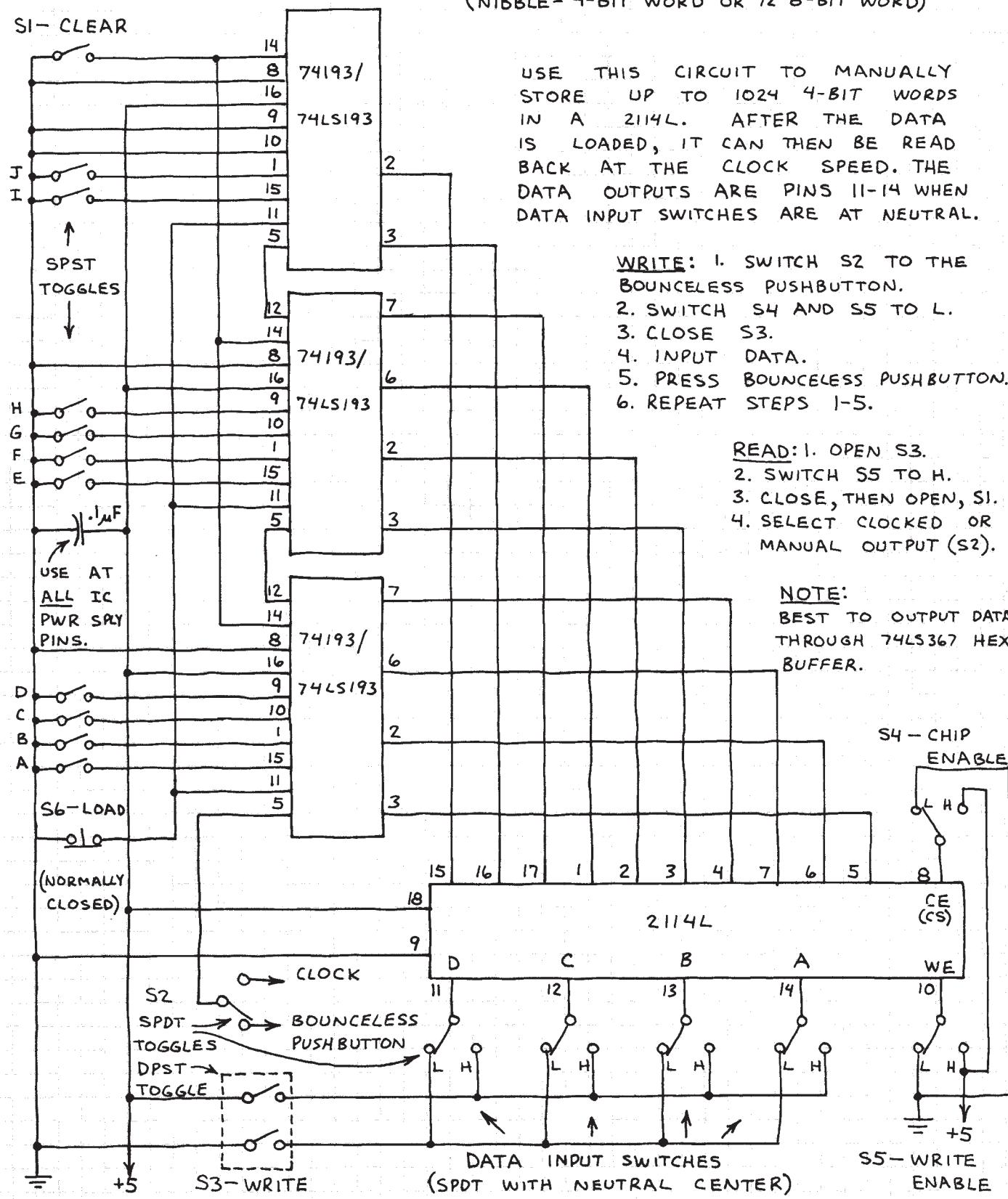
USE THIS CIRCUIT TO MANUALLY STORE UP TO 1024 4-BIT WORDS IN A 2114L. AFTER THE DATA IS LOADED, IT CAN THEN BE READ BACK AT THE CLOCK SPEED. THE DATA OUTPUTS ARE PINS 11-14 WHEN DATA INPUT SWITCHES ARE AT NEUTRAL.
