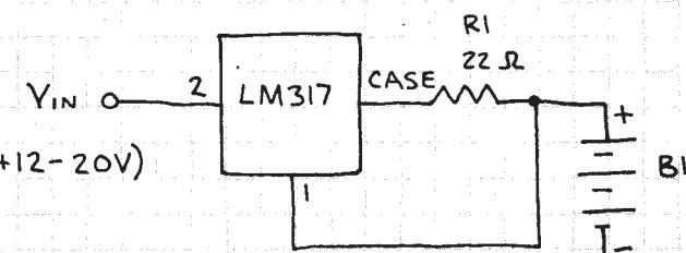
B1 IS BATTERY OF 4 NICKEL CADMIUM STORAGE CELLS IN SERIES. THIS CIRCUIT CHARGES B1 AT A CURRENT OF 51.2 mA. INCREASE R1 TO REDUCE CURRENT. FOR EXAMPLE, CURRENT IS 43 mA WHEN R1 IS 24 OHMS.
