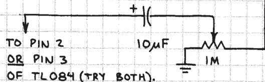
ADD THIS FEEDBACK CIRCUIT FOR UNUSUAL REVERBERATION EFFECTS. SLOW CLOCK FREQUENCIES GIVE MOST STRIKING REVERBERATIONS. TRY 5-20 kHz. FASTER CLOCK (20-100 kHz) AND CAREFUL ADJUSTMENT GIVES ROBOT-LIKE SOUND USED IN SOME SCIENCE FICTION MOVIES.
