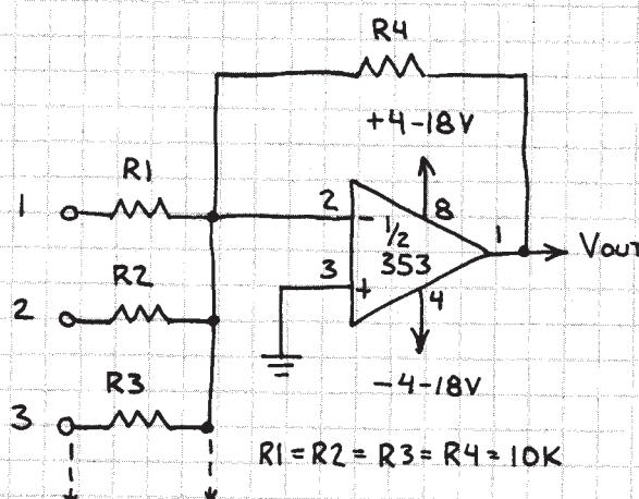
CONNECT OUTPUTS OF PREAMPLIFIERS TO INPUTS 1-3. OK TO ADD MORE CHANNELS. WORKS WELL WITH TL084 MICROPHONE PREAMPLIFIERS.
