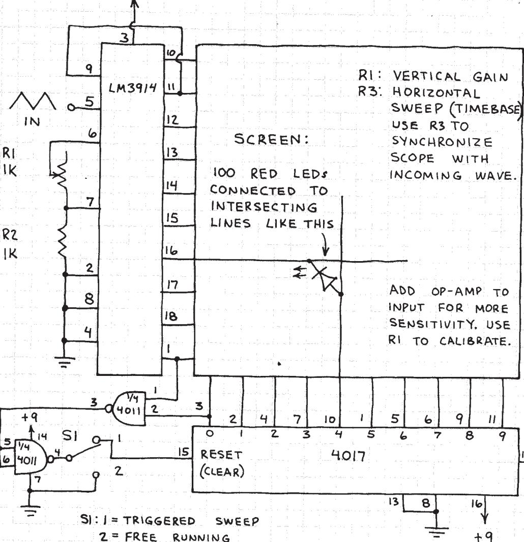
THIS IS AN EXPERIMENTAL SOLID-STATE SCOPE THAT WILL FIT IN A POCKET SIZE HOUSING. THE RESOLUTION IS POOR, BUT VARIOUS WAVEFORMS CAN BE VISUALIZED. EXPAND BOTH THE VERTICAL AND HORIZONTAL CIRCUITS FOR MORE RESOLUTION. FOR MORE INFORMATION SEE POPULAR ELECTRONICS, AUGUST 1979 (PP. 78-79).
