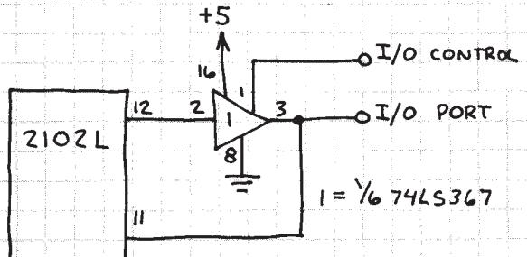
ADD THIS CIRCUIT TO THE ADDRESSING CIRCUIT ON FACING PAGE. WHEN I/O (INPUT/OUTPUT) CONTROL IS H, PIN 3 OF THE 74LS367 ENTERS THIRD STATE (HI-Z) AND I/O PORT ACCEPTS INPUT DATA. WHEN PIN 3 OF THE 74LS367 IS L, I/O PORT OUTPUTS DATA. BOTH THESE OPERATIONS ARE DEPENDENT UPON THE STATUS OF THE 2102L CONTROL INPUTS.
