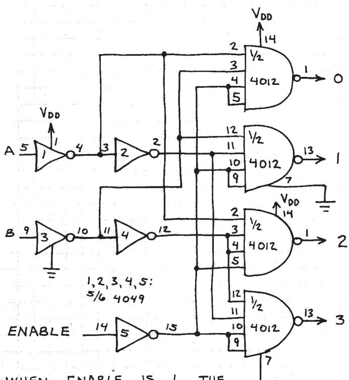
WHEN ENABLE IS L, THE OUTPUT CORRESPONDING TO THE BA BINARY INPUTS GOES LOW. ALL OTHER OUTPUTS GO HIGH WHEN ENABLE IS H.
