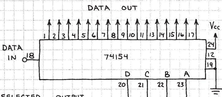
SELECTED OUTPUT IS LOW WHEN DATA IN IS LOW. IF DATA IN IS HIGH, SELECTED OUTPUT IS HIGH.
