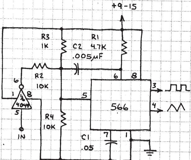
\* FSK MEANS FREQUENCY SHIFT KEYING.
