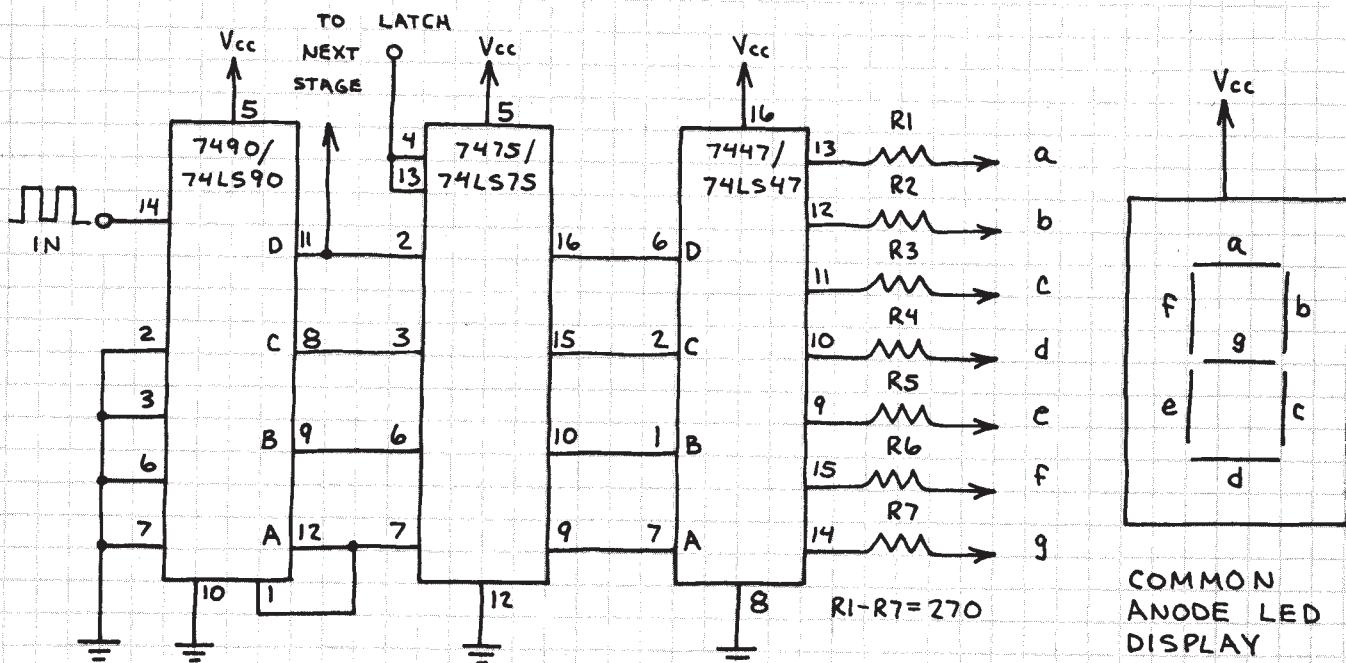
EXPANDABLE DECADE COUNTER. OF 7490/74LS90 OF FIRST UNIT TO INPUT OF SECOND UNIT. A LOW AT THE LATCH INPUT FREEZES THE DATA BEING DISPLAYED.
