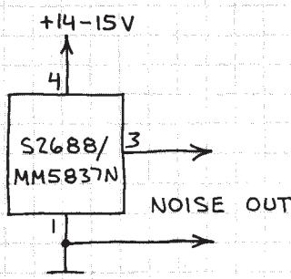
CONNECT OUTPUT TO AUDIO AMPLIFIER TO HEAR NOISE.
