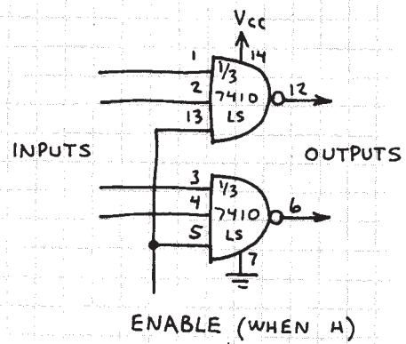
TYPICAL ENABLE INPUT CIRCUIT. USE THIS METHOD TO CONTROL ONE OR MORE GATES.
