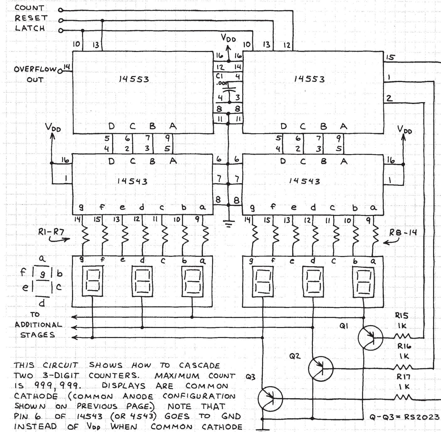
THIS CIRCUIT SHOWS HOW TO CASCADE TWO 3-DIGIT COUNTERS. MAXIMUM COUNT Q3 IS 999,999. DISPLAYS ARE COMMON CATHODE (COMMON ANODE CONFIGURATION SHOWN ON PREVIOUS PAGE). NOTE THAT PIN 6 OF 14543 (OR 4543) GOES TO GND INSTEAD OF V<sub>DD</sub> WHEN COMMON CATHODE DISPLAY IS USED.
