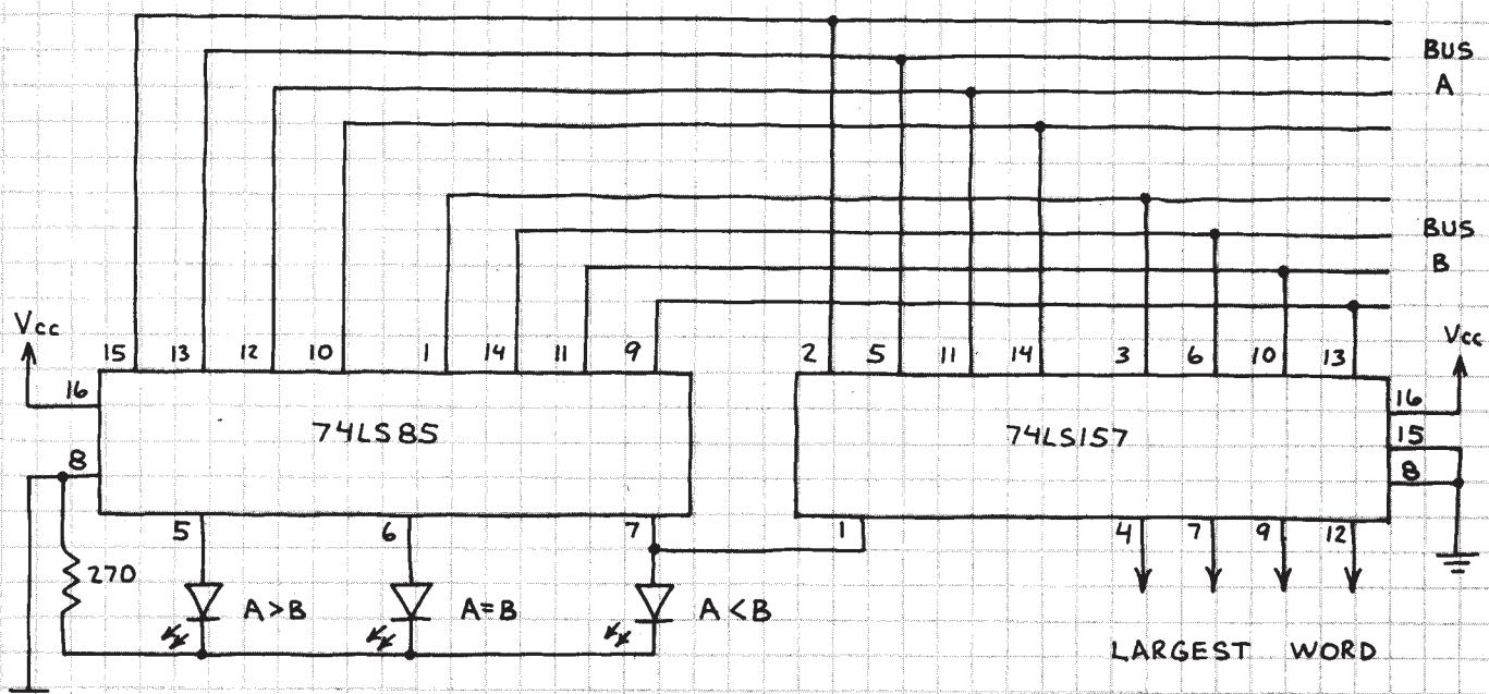
THIS CIRCUIT CONTINUALLY MONITORS TWO DATA BUSES. BUS WITH HIGHEST MAGNITUDE DATA WORD IS ROUTED AUTOMATICALLY TO OUTPUT.
