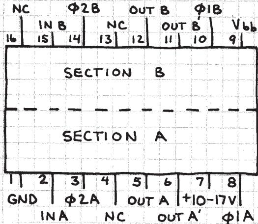
CAUTION: THIS NMOS CHIP IS VULNERABLE TO DAMAGE FROM STATIC DISCHARGE! FOLLOW CMOS HANDLING PROCEDURES.
