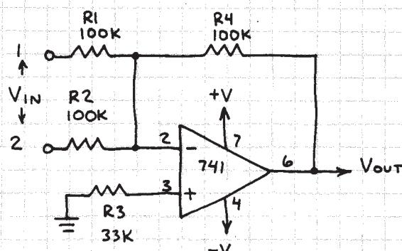
NOTE:  $V_{OUT}$  CANNOT EXCEED  $\pm V$ .
