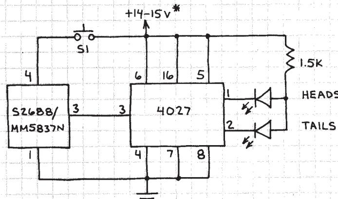
PRESS S1; BOTH LEDS GLOW. RELEASE S1 AND ONLY ONE GLOWS. GROUND INPUTS OF UNUSED HALF OF 4027 (PINS 9, 10, 11, 12 AND 13).\*(OK TO USE 9-VOLT BATTERY AS POWER SUPPLY.)
