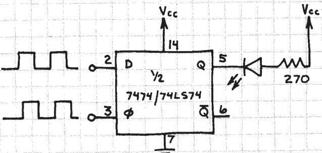
THE LED GLOWS WHEN INPUT FREQUENCIES  $F_1$  AND  $F_2$  ARE UNEQUAL OR OUT OF PHASE.  $F_1$  AND  $F_2$  SHOULD BE SQUARE WAVES.
