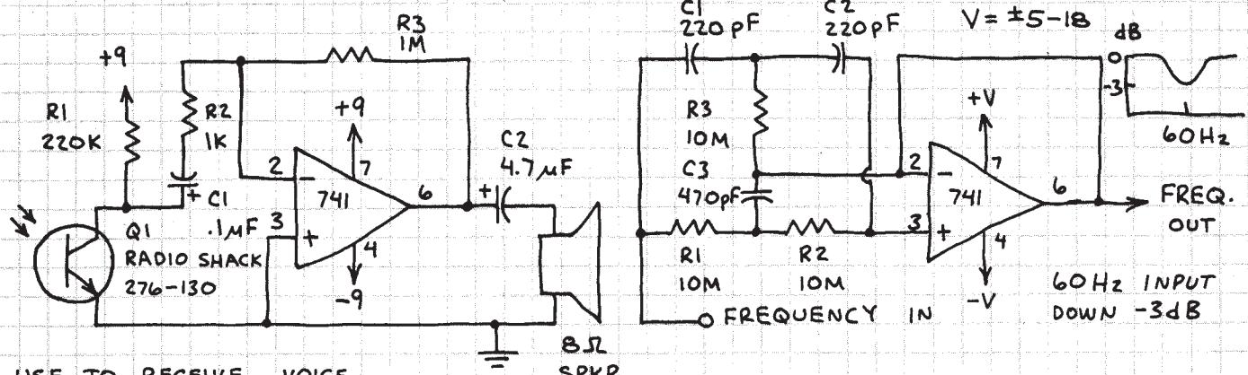
USE TO RECEIVE VOICE MODULATED LIGHT WAVES. OK TO USE SINGLE POLARITY POWER SUPPLY FOR NON-VOICE RECEPTION.
