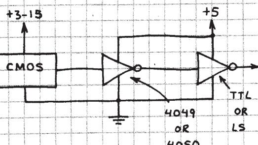
NOTE THAT CMOS MUST BE POWERED BY AT LEAST 5 VOLTS WHEN CMOS IS INTERFACED WITH TTL. OTHERWISE THE CMOS INPUT WILL EXCEED  $V_{dd}$ .
