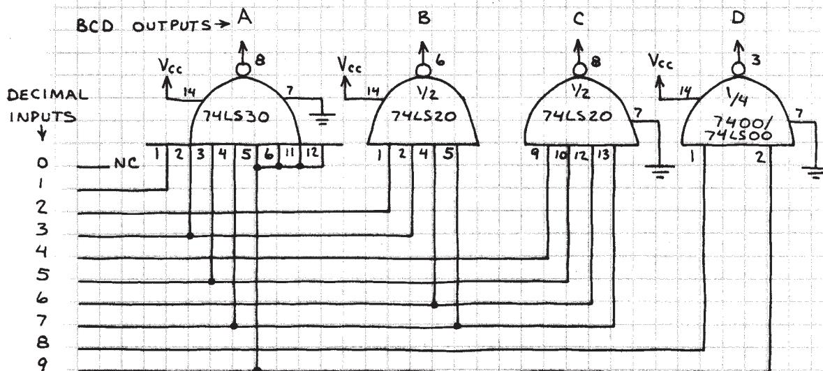
SELECTED INPUT SHOULD BE LOW AND ALL OTHER INPUTS SHOULD BE HIGH. BCD EQUIVALENT WILL APPEAR AT THE OUTPUTS.
