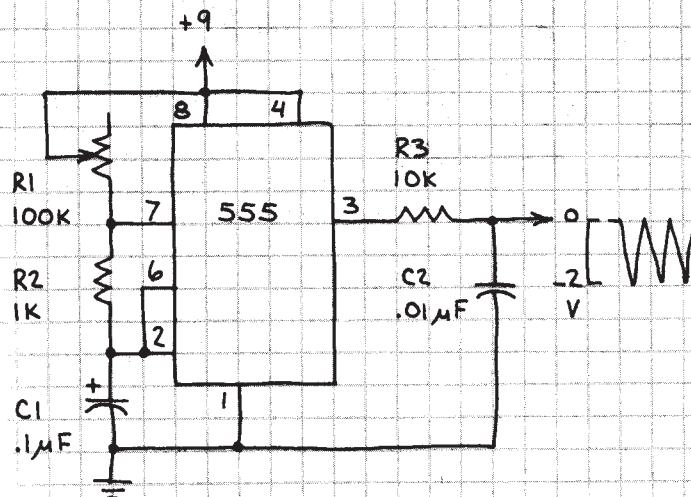
ADJUST R1 TO PROVIDE UP TO 10 kHz. OUTPUT FREQUENCY THIS HIGH PRODUCES CLOSELY SPACED TRIANGLE WAVES. THE WAVES ARE SEPARATED AT SLOWER FREQUENCIES (VVVV).
