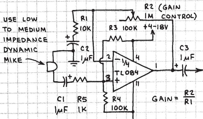
NOTE SINGLE POLARITY POWER SUPPLY (THANKS TO R3 AND R4) AND AC COUPLING.
