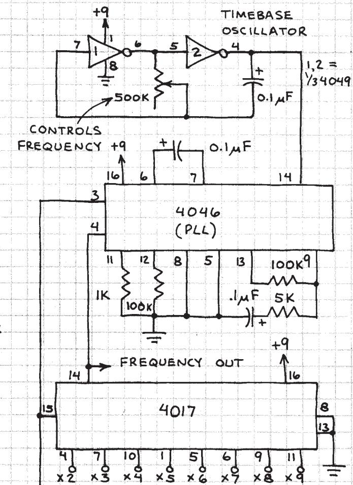
SELECT TIMEBASE FREQUENCY MULTIPLICATION FACTOR. SET TIMEBASE TO  $\sim 100$  Hz.
