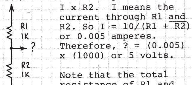
Note that the total resistance of  $R_1$  and  $R_2$  is simply  $R_1 + R_2$ . This rule provides a handy trick for making custom resistances.
