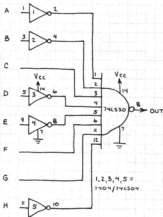
OUTPUT GOES LOW ONLY WHEN INPUT IS LHHLLHLL (DECIMAL 100). UP TO  $2^8$  INPUTS CAN BE DECODED BY REARRANGING UP TO 8 INPUT INVERTERS.
