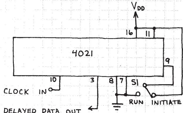
THE FIRST PARALLEL INPUT (PIN 7) IS GROUNDED. THIS LOADS A SINGLE L WHEN SI IS SWITCHED TO INITIATE. THE SINGLE L BIT REACHES THE OUTPUT AFTER 8 CLOCK PULSES.
