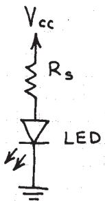
$$R_s = \frac{V_{CC} - V_{LED}}{LED_I}$$
