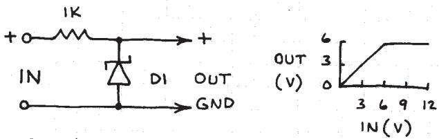
Zeners can also protect voltage sensitive components and provide a convenient reference voltage.
