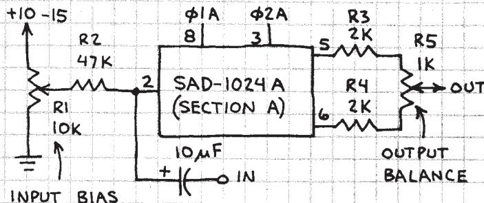
ADJUST  $R_1$  (INPUT BIAS) FOR OPTIMUM AUDIO OUTPUT. OUTPUTS APPEAR LIKE THIS ON A SCOPE:
