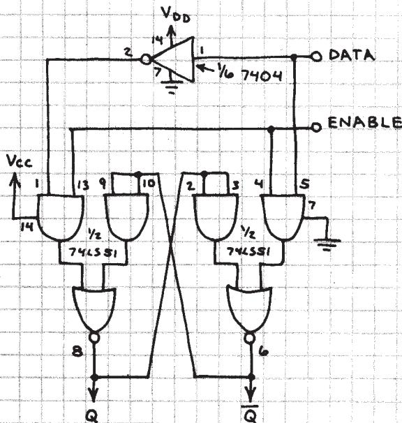
Q OUTPUT FOLLOWS DATA INPUT WHEN ENABLE INPUT IS HIGH. NO CHANGE WHEN ENABLE IS LOW.
