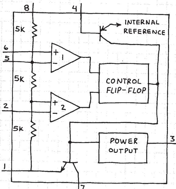
1 AND 2 ARE COMPARATORS. CIRCUIT CAN BE MADE FROM INDIVIDUAL PARTS AS SHOWN... BUT 555 IS MUCH SIMPLER.
