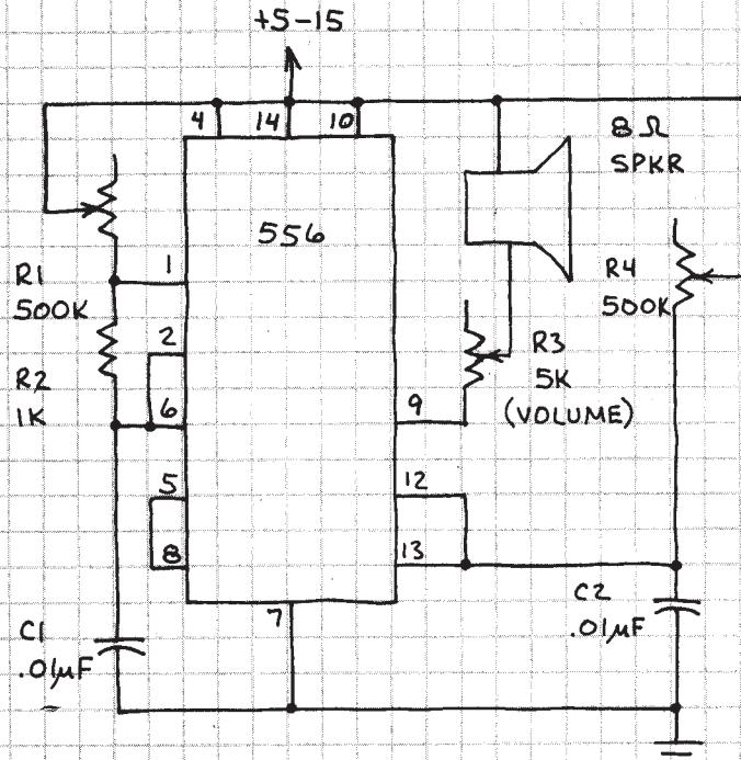
THIS CIRCUIT IS AN OSCILLATOR FOLLOWED BY A FREQUENCY DIVIDER. ADJUST R1 AND R4 FOR VERY UNUSUAL SOUND EFFECTS.
