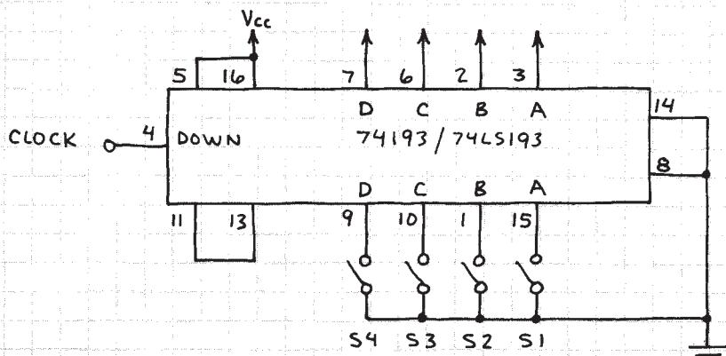
SET DESIRED N INTO S1-S4 (CLOSED SWITCH = LOW AND OPEN SWITCH = HIGH). WHEN COUNT REACHES LLLL AND THEN UNDERFLOWS, THE BORROW PULSE LOADS N AND THE COUNT RECYCLES.
