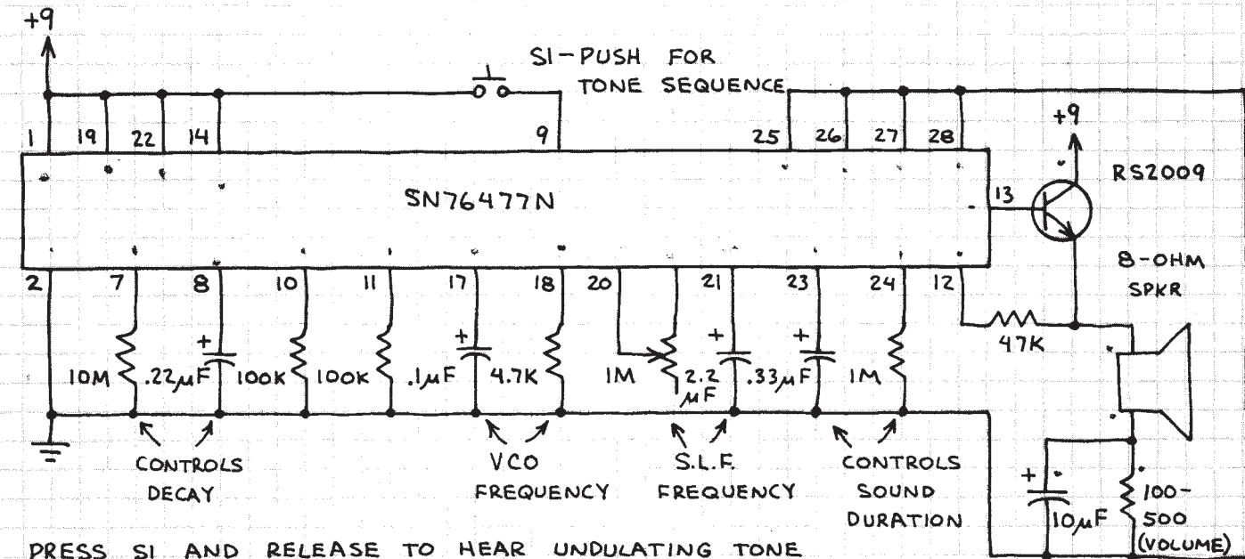
PRESS SI AND RELEASE TO HEAR UNDULATING TONE THAT GRADUALLY DECAYS AND STOPS. CHANGE VCO AND S.L.F. COMPONENTS FOR MANY DIFFERENT SOUND EFFECTS RANGING FROM SIREN TO SCIENCE FICTION MOVIE SOUNDS. FOR CONTINUOUS SOUND, OMIT COMPONENTS AT PINS 7, 8, 23, 24 AND GROUND PIN 9.
