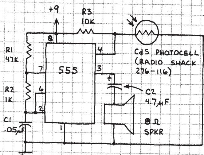
SILENT WHEN LIGHT STRIKES PHOTOCELL. REMOVE LIGHT AND TONE SOUNDS. FASTER RESPONSE THAN ADJACENT CIRCUIT.
