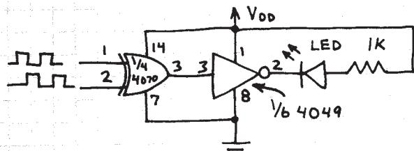
LED STOPS GLOWING WHEN THE INPUT FREQUENCIES ARE EQUAL.
