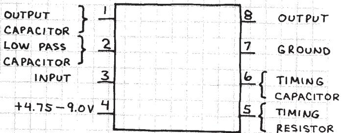
THE VALUE IN MICROFARADS OF THE LOW PASS CAPACITOR SHOULD BE  $n/f_0$  WHERE n RANGES BETWEEN 1300 (FOR UP TO 14%  $f_0$  DETECTION BANDWIDTH) TO 62,000 (UP TO 2%  $f_0$  DETECTION BANDWIDTH). THE OUTPUT CAPACITOR SHOULD HAVE ABOUT TWICE THE CAPACITANCE OF THE LOW PASS FILTER CAPACITOR.
