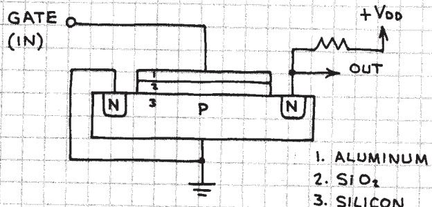
A PMOS TRANSISTOR IS IDENTICAL EXCEPT THE P AND N REGIONS ARE EXCHANGED. THE  $\text{SiO}_2$  (SILICON DIOXIDE) LAYER IS A GLASSY FILM THAT SEPARATES AND INSULATES THE METAL GATE FROM THE SILICON SUBSTRATE. THIS FILM IS WHY A MOS TRANSISTOR OR IC PLACES PRACTICALLY NO LOAD ON THE SOURCE OF AN INPUT SIGNAL. THE FILM IS VERY THIN AND IS THEREFORE EASILY PUNCTURED BY STATIC ELECTRICITY:
