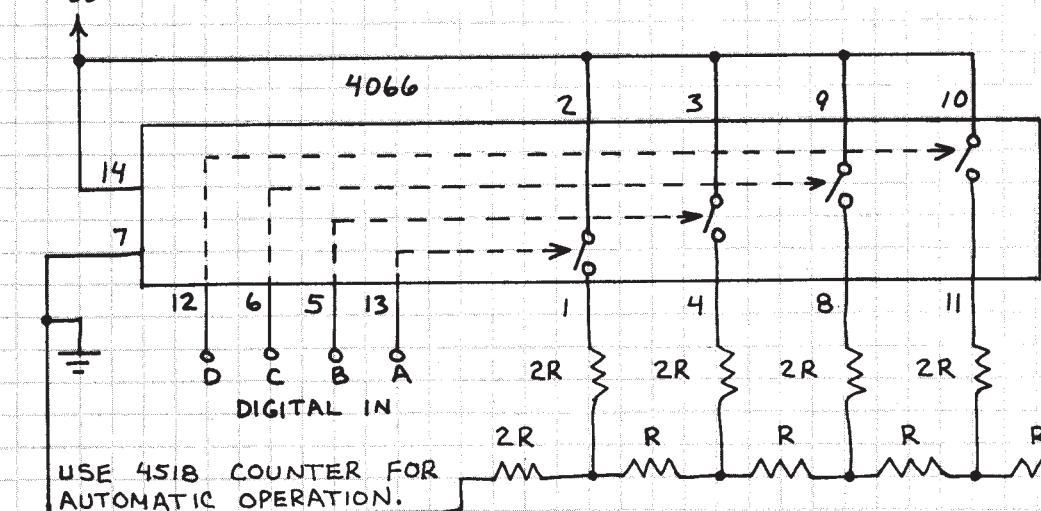
THIS IS NOT A LINEAR D/A CONVERTER. INSTEAD IT PRODUCES A PSEUDO-RANDOM OUTPUT THAT RANGES FROM 3.06 - 5.62 VOLTS ( $V_{DD} = 9$  V). USE TO DRIVE 4046 VCO OR PRODUCE UNUSUAL WAVEFORMS.  $R = 47K$  AND  $2R = 100K$ .
