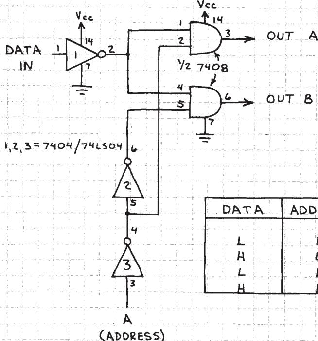
THIS CIRCUIT STEERS THE INPUT BIT TO THE OUTPUT SELECTED BY THE ADDRESS.
