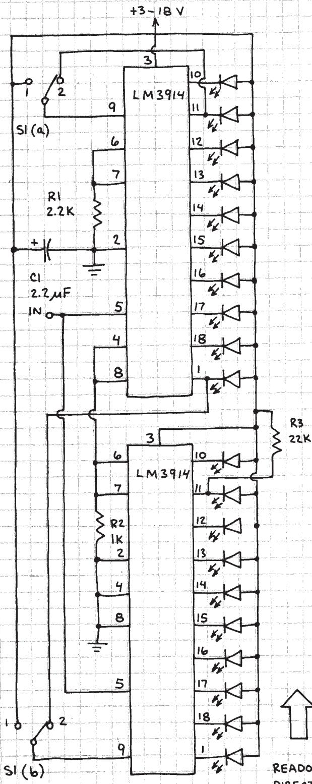
THIS CIRCUIT SHOWS HOW TO CASCADE 2 OR MORE LM3914'S. WHEN  $+V = 5$  VOLTS, THE READOUT RANGE IS 0.14 V TO 2.7 V. HIGHEST ORDER LED STAYS ON DURING OVERRANGE. AVOID SUBSTITUTIONS FOR R<sub>1</sub>, R<sub>2</sub> AND R<sub>3</sub>.
