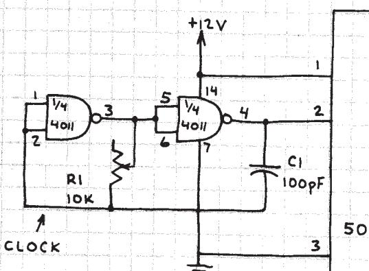
FOR TOP OCTAVE, ADJUST R1 FOR CLOCK FREQUENCY OF 2.00024 MHz. FOR NEXT LOWER OCTAVE, USE 1.00012 MHz CLOCK FREQUENCY.
