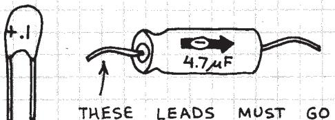
Capacitors have a voltage rating. It's usually printed under the capacity marking. The voltage rating must be higher than the highest expected voltage (usually the power supply voltage).
