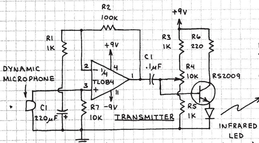
POINT THE LED AT Q1 AND ADJUST R4 UNTIL BEST VOICE QUALITY IS OBTAINED. (R4 APPLIES PREBIAS TO LED.) R6 LIMITS MAXIMUM LED CURRENT TO A SAFE 40 mA.
