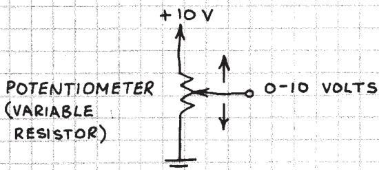
And they're useful in voltage sensing circuits. See the comparator circuits in this notebook.
