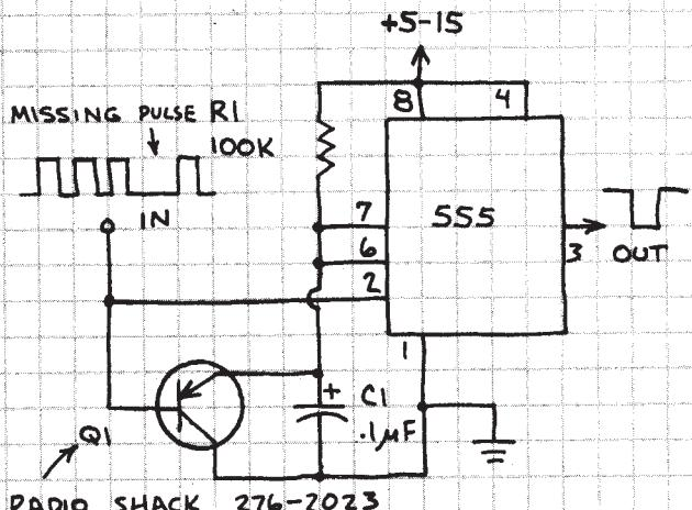
THIS CIRCUIT IS A ONE-SHOT THAT IS CONTINUALLY RETRIGGERED BY INCOMING PULSES. A MISSING OR DELAYED PULSE THAT PREVENTS RETRIGGERING BEFORE A TIMING CYCLE IS COMPLETE CAUSES PIN 3 TO GO LOW UNTIL A NEW INPUT PULSE ARRIVES. R1 AND C1 CONTROL RESPONSE TIME. USE IN SECURITY ALARMS, CONTINUITY TESTERS, ETC.
