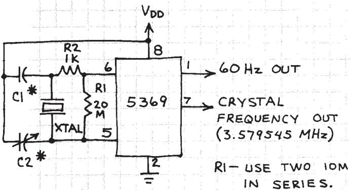
\* MOTOROLA SPECIFIES THAT  $C_1 = 30\text{ pF}$  AND  $C_2 = 6.36\text{ pF}$ . OK TO USE SIX  $4.7\text{ pF}$  CAPACITORS IN PARALLEL OR  $47\text{ pF}$  CAPACITOR FOR  $C_1$ . TRY TUNABLE CAPACITOR (e.g.  $5-50\text{ pF}$ ) FOR  $C_2$ . TO TUNE, CONNECT FREQUENCY METER TO PIN 7. TUNE  $C_2$  UNTIL FREQUENCY IS 3,579,545 Hz. ACCURACY FAIRLY GOOD EVEN IF YOU DON'T TUNE  $C_2$ .
