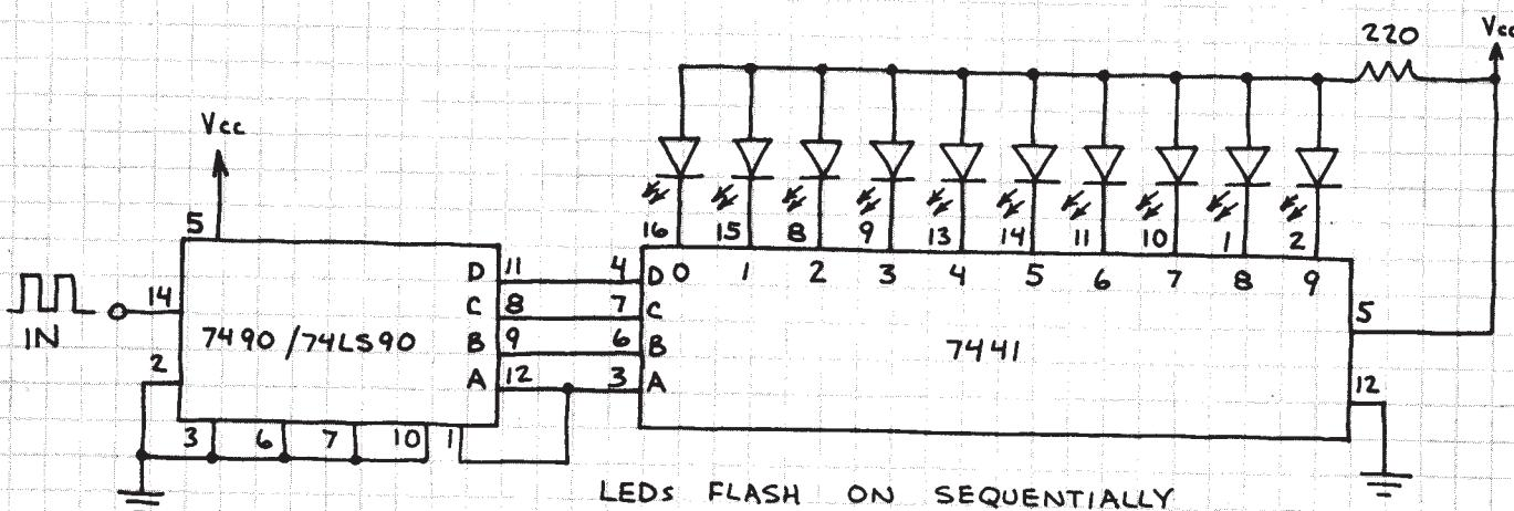
LEDS FLASH ON SEQUENTIALLY IN RESPONSE TO DECODED COUNT. ONLY ONE LED SERIES RESISTOR IS REQUIRED.
