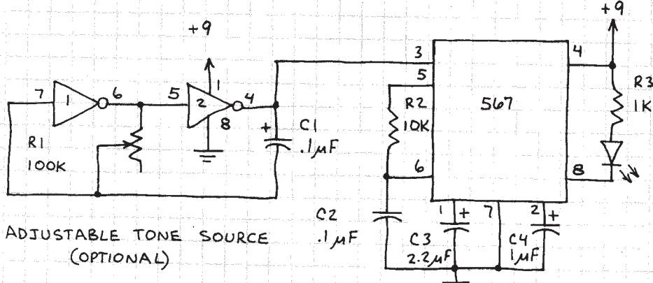
THIS CIRCUIT IS HANDY FOR LEARNING TONE DECODER BASICS. THE 567 PORTION CAN BE USED IN MANY DIFFERENT APPLICATIONS (SEE BELOW). THE PREDICTED  $f_0$  IS 1.1 kHz. THE TEST CIRCUIT  $f_0$  WAS 1.3 kHz.
