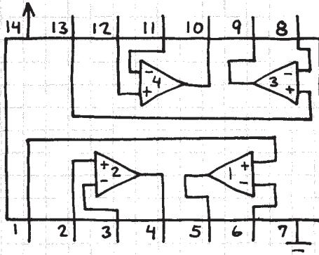
OPERATES FROM SINGLE POLARITY POWER SUPPLY. LESS GAIN (70 dB) BUT WIDER BANDWIDTH (25 MHz AT GAIN OF 1) THAN THE LM324 QUAD OP-AMP. NOTE STANDARD POWER SUPPLY PIN LOCATIONS. CAUTION: SHORTING THE OUTPUTS DIRECTLY TO V<sub>T</sub> OR GROUND OR REVERSED POWER CONNECTIONS MAY DAMAGE THIS CHIP.
