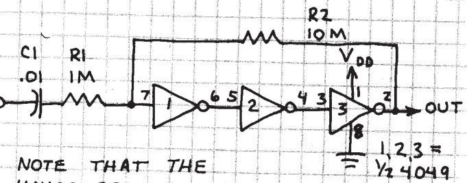
NOTE THAT THE INVERTERS ARE USED IN A LINEAR MODE. GAIN =  $R_2/R_1$ .
