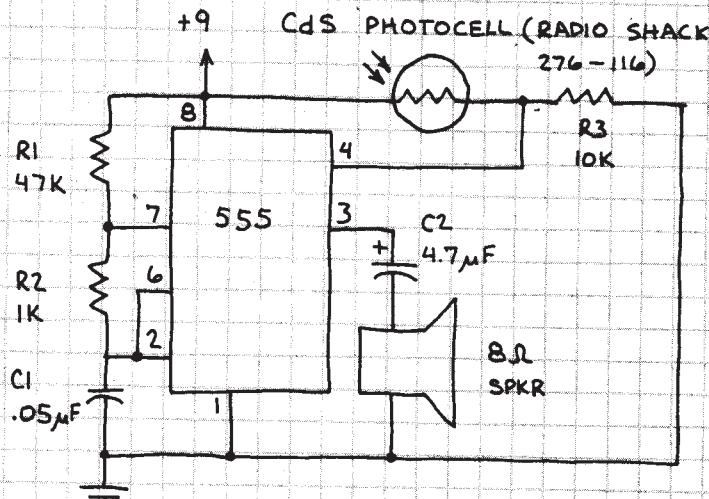
PRODUCES WARNING TONE WHEN LIGHT STRIKES PHOTOCELL. MAKES A GOOD OPEN DOOR ALARM FOR REFRIGERATOR OR FREEZER.
