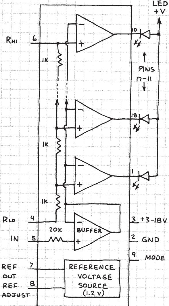
R<sub>H1</sub> AND R<sub>LO</sub> ARE THE ENDS OF THE DIVIDER CHAIN. THE REFERENCE VOLTAGE OUTPUT (REF OUT) IS 1.2-1.3 VOLTS. CONNECT PIN 9 TO PIN 11 FOR DOT MODE OR +V FOR BAR MODE.
