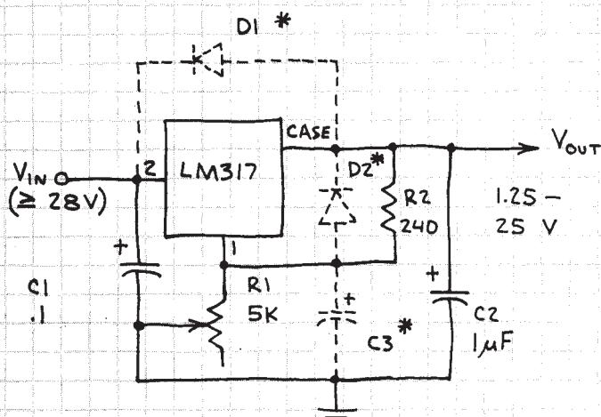
V<sub>IN</sub> SHOULD BE FILTERED. OK TO OMIT C1 IF V<sub>IN</sub> VERY CLOSE TO LM317.
