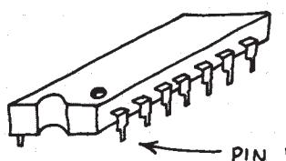
When the IC is right side up, pin 1 is at lower left:
