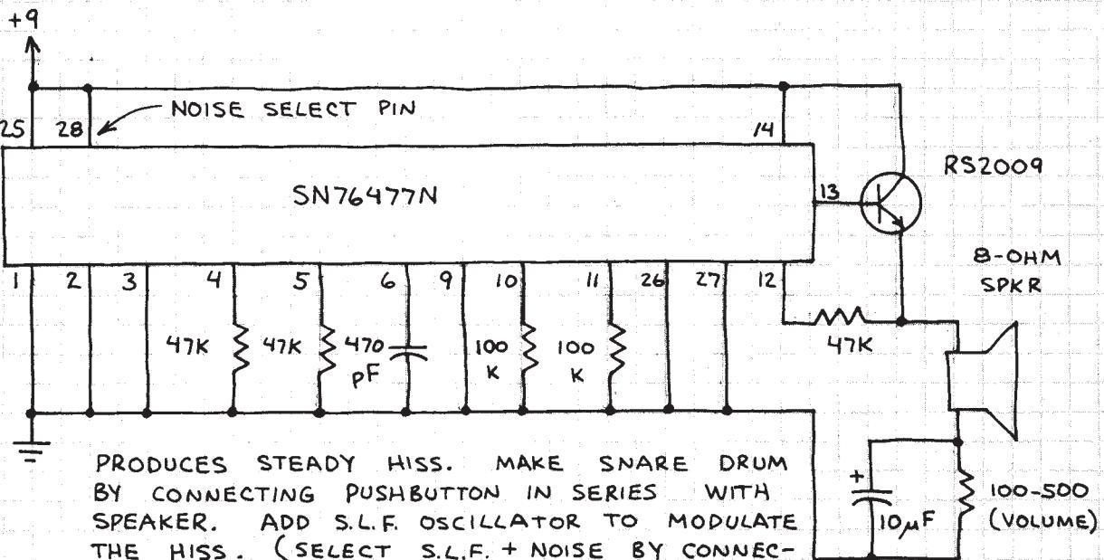
PRODUCES STEADY HISS. MAKE SNARE DRUM BY CONNECTING PUSHBUTTON IN SERIES WITH SPEAKER. ADD S.L.F. OSCILLATOR TO MODULATE THE HISS. (SELECT S.L.F. + NOISE BY CONNECTING PINS 25 AND 26 TO GND AND PIN 27 TO +9V. ADD 1M POT FROM PIN 20 TO GND AND 1μF CAPACITOR FROM PIN 21 TO GND.) SOUNDS LIKE STEAM TRAIN OR PROPELLER AIRCRAFT DEPENDING ON ADJUSTMENT OF 1M POT.
