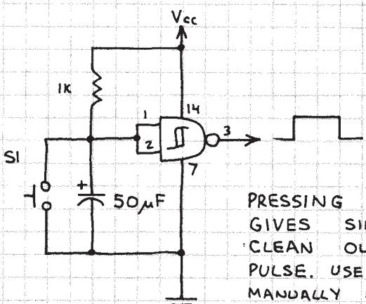
PRESSING SI GIVES SINGLE, CLEAN OUTPUT PULSE. USE FOR MANUALLY INJECTING LOGIC SIGNALS, ETC.
