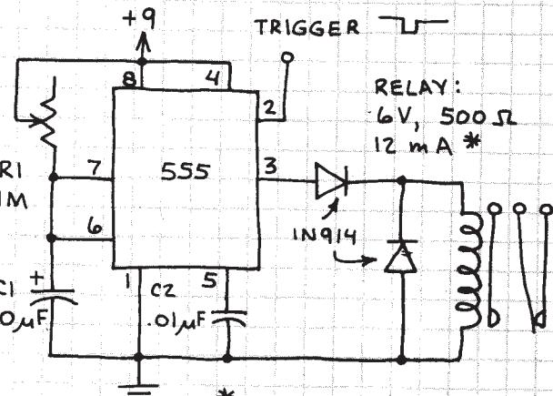
VALUES OF R1 AND C1 SHOWN WILL PULL RELAY IN FOR UP TO ABOUT 11 SECONDS. USE POINTER KNOB AND PAPER SCALE TO HELP CALIBRATE CIRCUIT. USES INCLUDE DARKROOM TIMING. CIRCUIT CAN BE TRIGGERED BY A NEGATIVE PULSE OR WITH A PUSHBUTTON SWITCH ACROSS PINS 1 AND 2.
