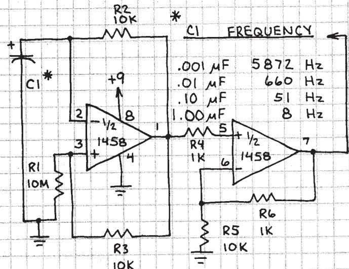
PULSES ARE DC. AMPLITUDE WHEN  $C_1 = 0.1 \mu F$  IS 5 VOLTS.
