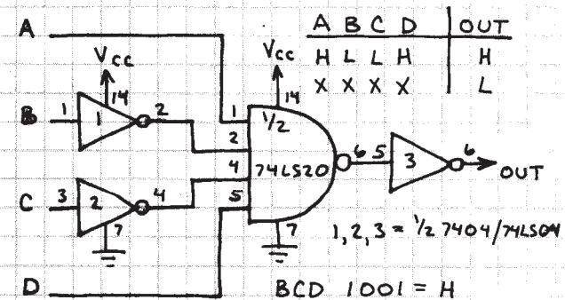
OUTPUTS GO HIGH WHEN APPROPRIATE BCD WORD APPEARS AT INPUTS DCBA. OUTPUTS STAY LOW FOR ALL OTHER INPUTS. (OMIT FINAL INVERTER TO PROVIDE ACTIVE LOW OUTPUT.) USE THIS METHOD TO DECODE ANY 4-BIT NIBBLE.
