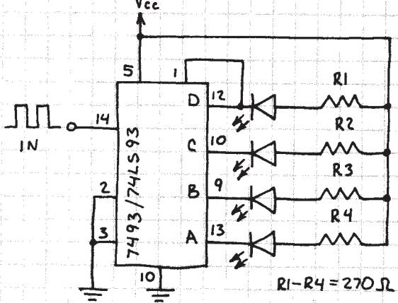
COUNTS FROM 0-15 IN BINARY AND RECYCLES. GLOWING LED = L (0); OFF LED = H (1). 555 TIMER IC MAKES GOOD INPUT CLOCK.
