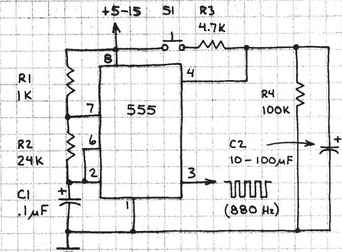
PRESS S1 AND STEADY OUTPUT FREQUENCY APPEARS AT PIN 3. RELEASE S1 AND OUTPUT FREQUENCY CONTINUES UNTIL C2 IS DISCHARGED BY R4. INCREASE C2 (OR R4) TO INCREASE LENGTH OF THE BURST. CHANGE FREQUENCY OF TONE BURST VIA R2 OR C1.
