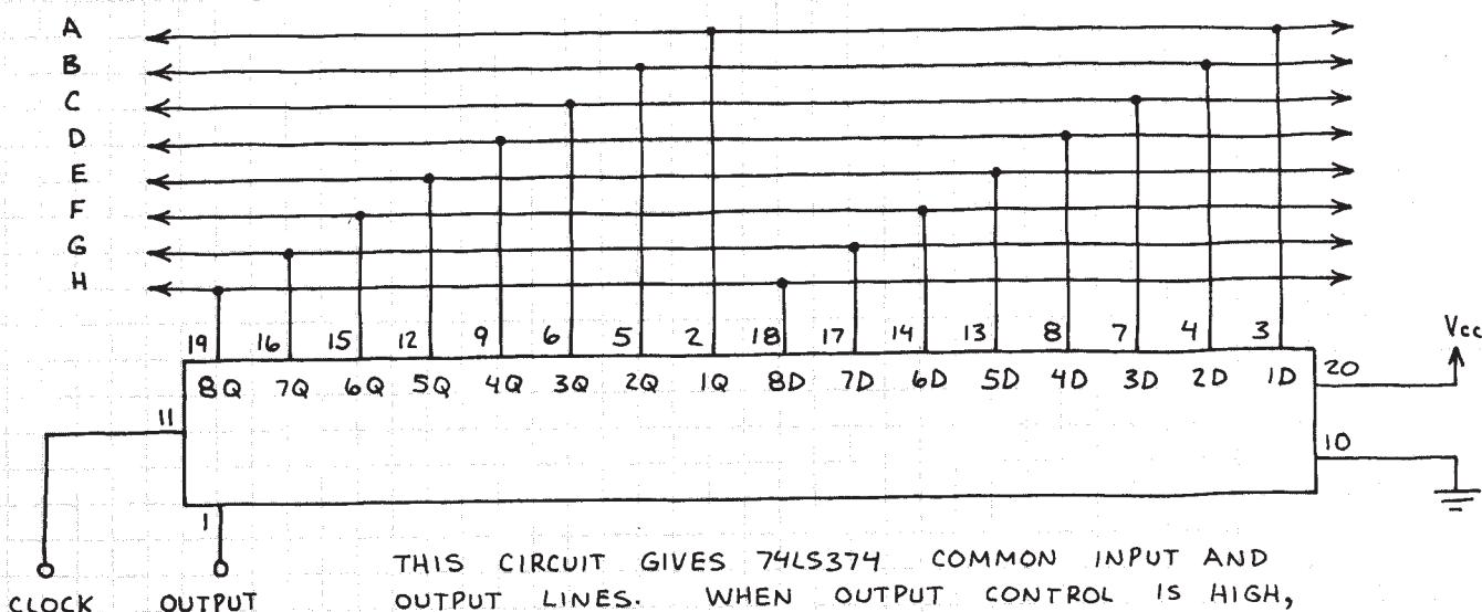
THIS CIRCUIT GIVES 74LS374 COMMON INPUT AND OUTPUT LINES. WHEN OUTPUT CONTROL IS HIGH, DATA ON BUS IS LOADED INTO THE 74LS374 ON THE RISING EDGE (↑) OF THE CLOCK PULSE. WHEN OUTPUT CONTROL IS LOW, DATA IN THE 74LS374 IS WRITTEN ONTO THE BUS.
