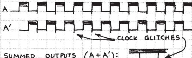
SET SCOPE TO VISUALIZE INPUT SIGNAL (COMPRESSING CLOCK RATE):
