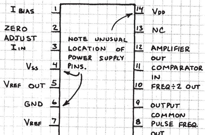
CAUTION: THIS CHIP INCORPORATES BOTH BIPOLAR AND CMOS CIRCUITRY. THEREFORE CMOS HANDLING PRECAUTIONS MUST BE FOLLOWED TO AVOID PERMANENT DAMAGE.
