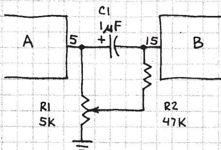
$R_1$  CONTROLS BIAS TO SECTION B. NOTE THAT ONLY ONE OUTPUT OF A IS CONNECTED TO INPUT OF B.
