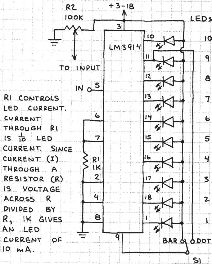
WHEN +V = +3-18 VOLTS, THE READOUT RANGE IS 0.13 - 1.30 VOLTS. TO CHANGE RANGE TO 0.1-1.0 VOLT (0.1 VOLT PER LED), INSERT A 5K POTENTIOMETER BETWEEN PINS 6 AND 7. CONNECT VOLTMETER ACROSS PINS 5 AND 8 AND ADJUST R2 FOR 1 VOLT AT PIN 5. THEN ADJUST 1K POT UNTIL LED 10 GLOWS. REPEAT THIS PROCEDURE FOR 0.1 VOLT AT PIN 5 AND LED 1. OK TO REPLACE THE 1K POT WITH A FIXED RESISTOR OF THE PROPER VALUE.
