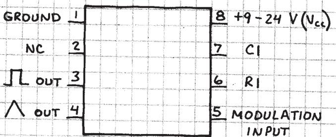
$$\text{CENTER FREQUENCY} = \frac{2(V_{cc} - \text{INPUT VOLTS})}{R_1 C_1 V_{cc}}$$
