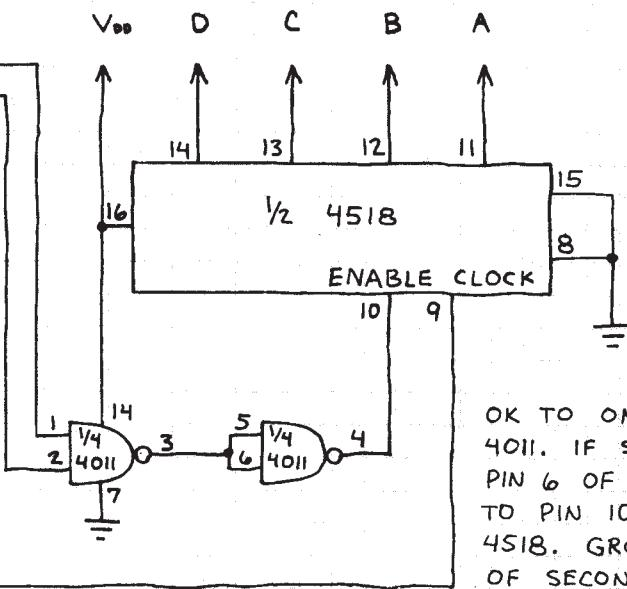
OK TO OMIT THE 4011. IF SO, CONNECT PIN 6 OF FIRST 4518 TO PIN 10 OF SECOND 4518. GROUND PIN 9 OF SECOND 4518 AND APPLY INPUT TO PIN 1 OF FIRST 4518.
