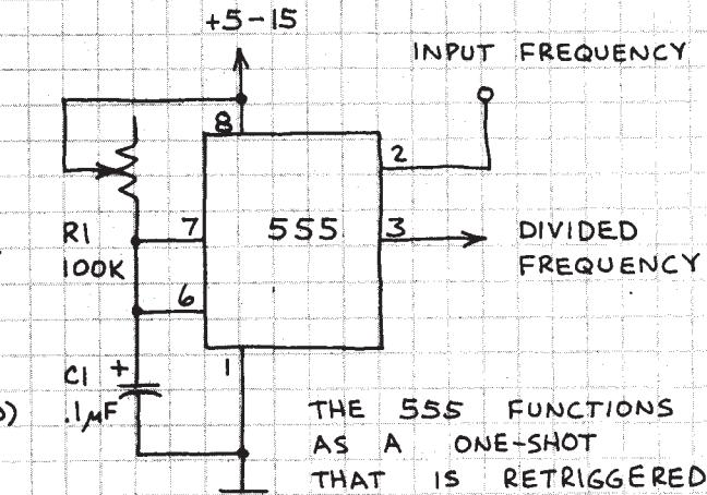
THE 555 FUNCTIONS AS A ONE-SHOT THAT IS RETRIGGERED BY THE INPUT WAVE. WAVES ARRIVING DURING THE TIMING CYCLE ARE IGNORED.
