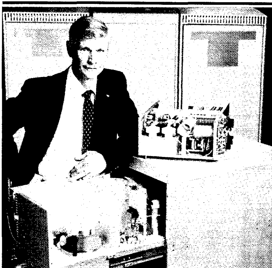
Dick Ehrhorn with ETO’s latest 20-kW MRI amplifier and to his left, an Alpha 86 amp. Visible in the pull-out drawer is the MRI’s RF deck with its final, a modified Eimac 3CX15000B7. A solid-state 300-watt exciter drives a 3CX800 that drives the big tube. The power supply is below the RF deck.
